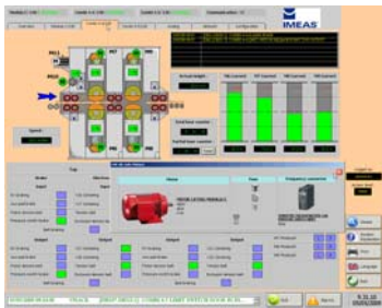
Sanding machine details w/motor load
